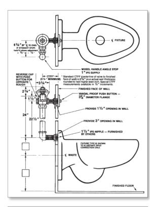
Recommended For: Penal or heavier duty installations where vandalism and abuse are common. No parts of valve can be removed from front face of wall. Access to rear of wall for future service of valve and vacuum breaker must be provided.
