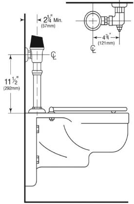
**Note:** Min.roughing height 10 1/2" centerline of supplu to top of fixture.
